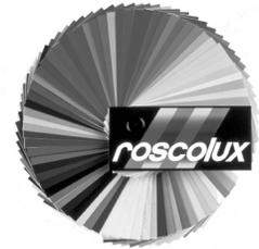
Stage lighting is usually colored by placing a thin sheet of plastic in front of the lens. These sheets are called “color filters,” or “gel” because they were originally made of dyed animal gelatin. Modern gel has a polymer base of acetate, vinyl, polyester or polycarbonate. Stage lighting fixtures produce very high temperatures and the light filtered by the gel is converted to heat. Therefore, do not use anything except color filters designed for use in entertainment lighting.
